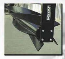
Spiral crumbler ridges or checks field surface to improve pre-irrigation and crimps crop residue into soil
