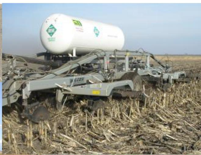
**Chassis' 10,000 lb. carrying capacity not only affords the "new seeding" attachment, but also allows for fertilizer and herbicide tanks.**
